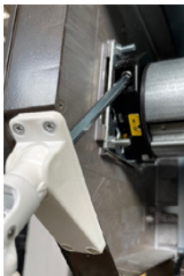
If a 45° box is not fitted, secure the knuckle to the endplate flange.
